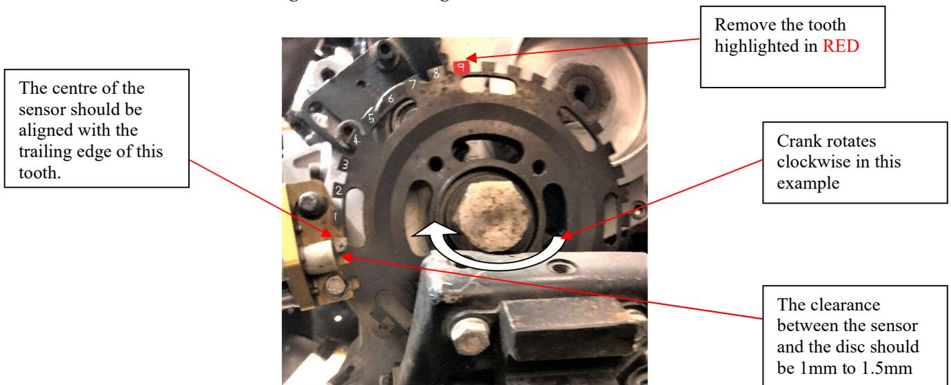
Small amounts ( $\pm 5$  degrees) of misalignment can be corrected with the offset adjustment in the PC software.
