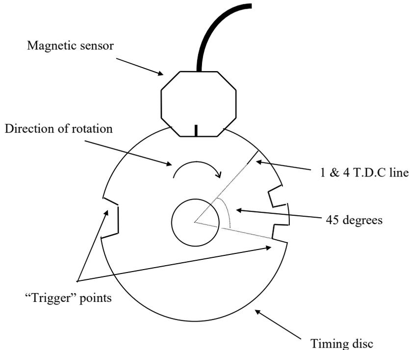
**Figure 3. POLESTAR Timing Disc and Sensor Alignment (multi-coil)**
