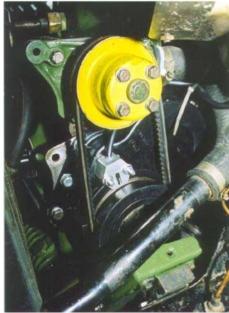
**Figure 2 Typical Sensor Fitting on A-Series Engine**
