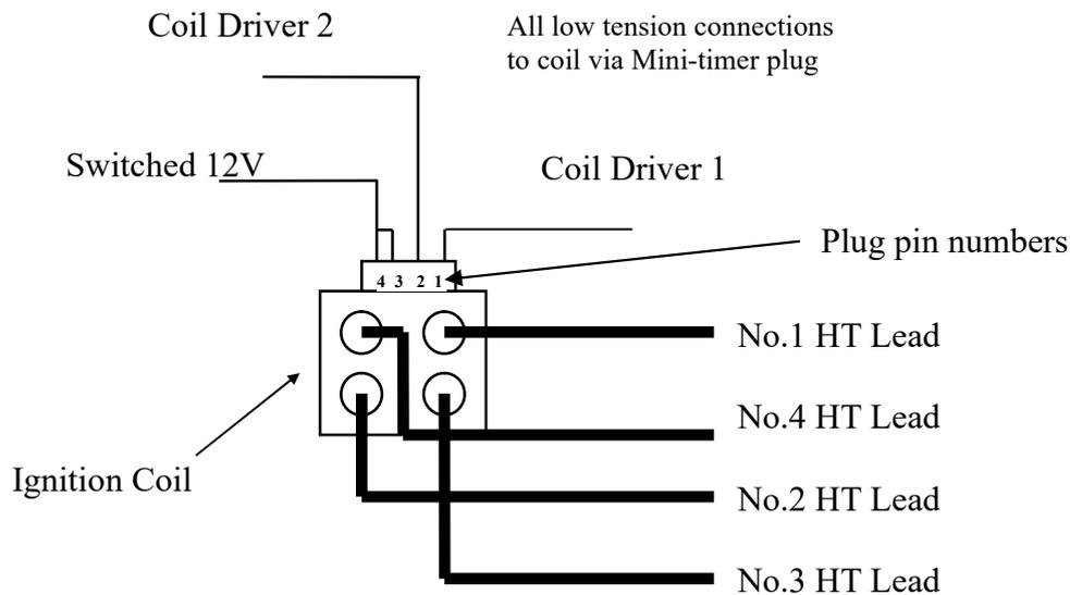
Another possible coil is that as fitted to a 1995 Ford Fiesta (or equivalent). There is an old Ford part number of 928F12029CA, but there are equivalents around such as the CAMBIARE VE520051 which works very well. This coil has three low tension connections and four high tension outputs each of which connect via an ignition lead to a spark plug (see Figure 5). CAMBIARE also supply some quality HT ignition leads for this coil part number VE522125.
