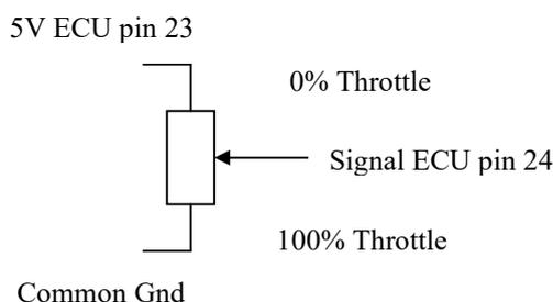
Figure 6 shows the correct wiring of the throttle sensor.
