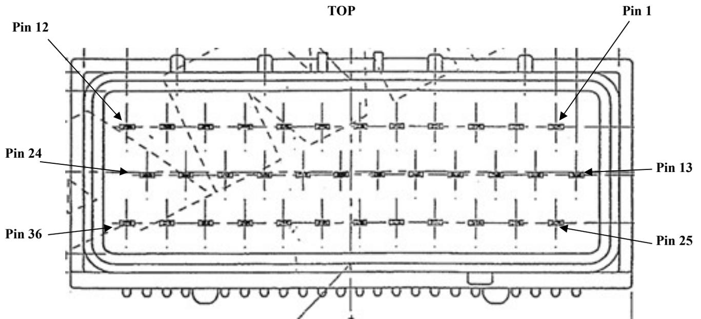
The above diagram indicates the pin numbering looking into the connector on the end of the ECU.
